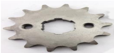
Gambar 1. Roda Gigi Tarik Spedea Motor
