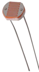
Gambar 2. Sensor Cahaya LDR ( Light Dependent Resistor )
