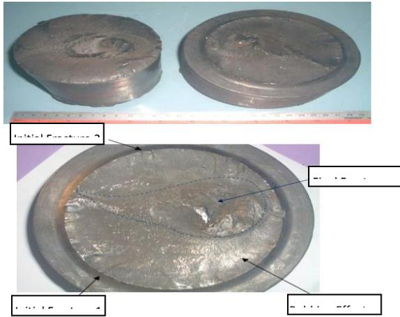
Figure 4. The fracture surface because of rotating bending
