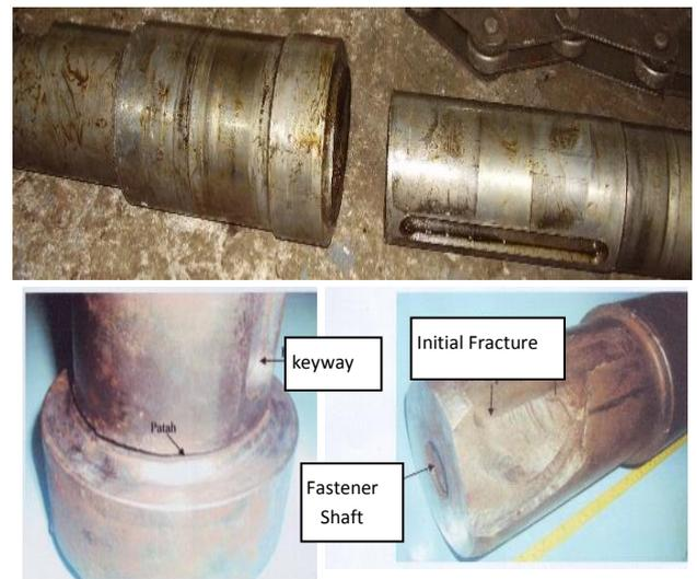
Figure 3. The fracture of screw press of the drive shaft
