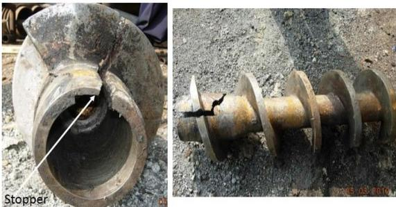
Figure 5. Worm screw damaged
